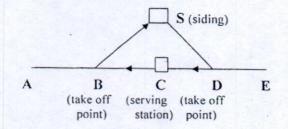
In this case, traffic is coming from station E and B & D are two take off points on both side of the serving station C. However, if due to some problem in DS route for which siding owner is responsible, the traffic goes via C and B to siding S, the chargeable distance will be equal to distance upto E plus distances from E to C, C to B and B to S. However, if the route
