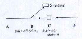
The traffic coming from side D which is a junction station passes through serving station C and goes to siding via B, the take off point. The chargeable distance will be equal to distance upto C plus distances from C to B and from B to siding S.
