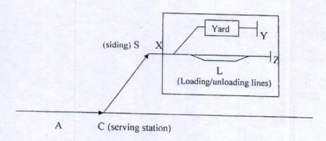
L denotes loading/unloading lines, Y is the buffer end of yard, X is common entry point for both yard & loading/unloading lines and Z is buffer end of siding.
