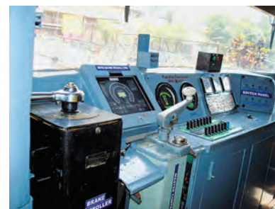
Train Protection and Warning System (TPWS) installed in EMU/MEMU, SR
