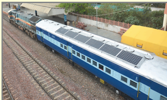
Coach with Rooftop Solar Panel
