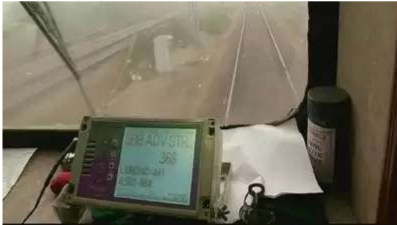
Fig. 2: Fog Safe device being used in train
