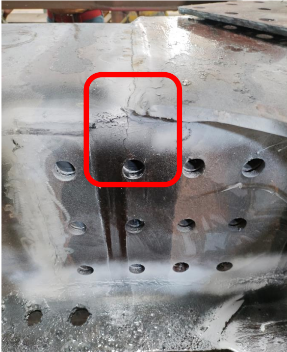
Crack in web of Centre Sill below Centre Sill - Bolster top plate joint.
