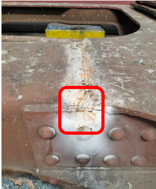
Crack/failure of weld joint between Centre Sill top & Bolster top plate, crack also initiate & propagate in Knee plate.
