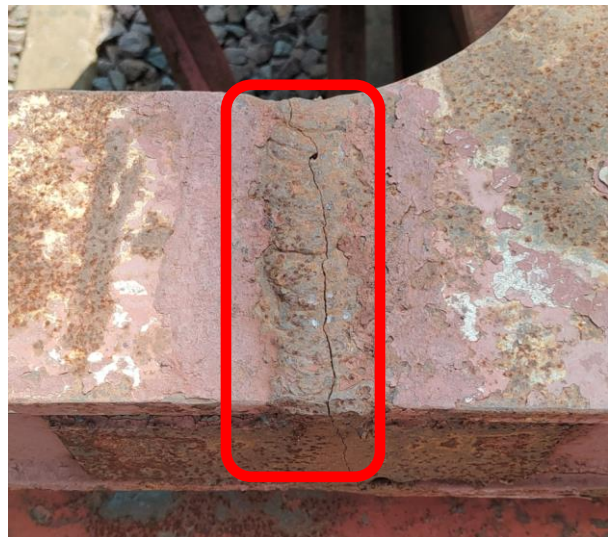
Weld crack/failure at joint between top plates of Solebar & Bolster sub-assemblies
