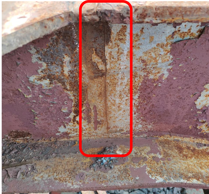
Crack in web plate of Centre Sill-Middle at joint between Centre Sill top plate and Bolster top plate
