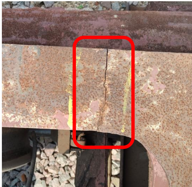
Weld crack/failure at joint between top plates of Solebar & Bolster sub-assemblies
