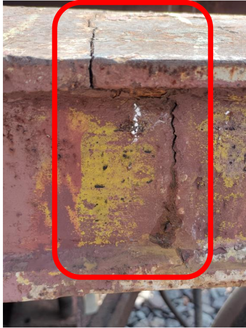
Weld crack/failure at joint between web plate of Solebar & Bolster sub-assemblies
