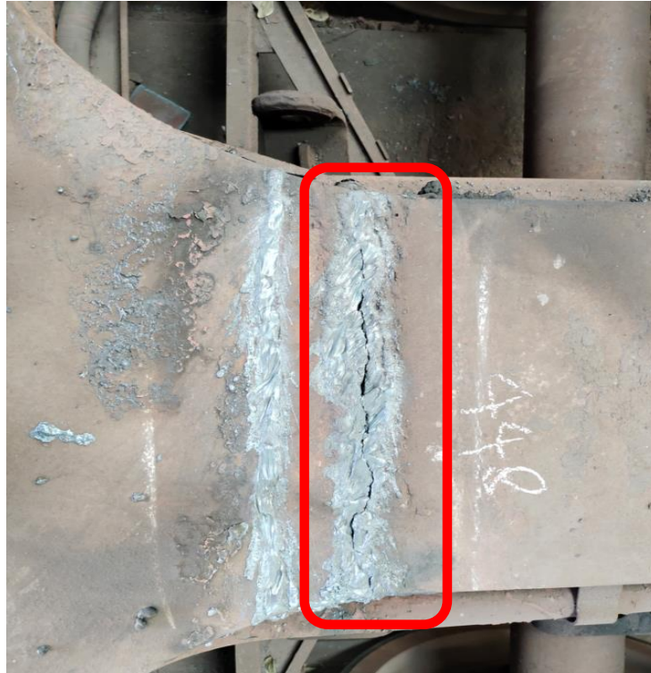
Centre Sill (towards Headstock) - Bolster top plate weld joint failure
