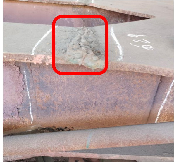
Centre Girder (Centre Sill-Middle) Top plate - Bolster Top plate weld joint failure
