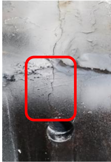
Crack in web of Centre Sill below Centre Sill - Bolster top plate joint.
