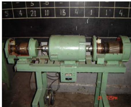
3. Two nos. self Mounted Traction Alternator was modified into conventional type, as the Traction Alternator received from DLW does not contain inbuilt self-Mounted Rectifier. The requirement of Traction Alternator was met by modification of self Mounted Traction Alternator into conventional type and it fitted over the locomotive. All these modification were possible by dedicated effort of Traction Motor section staff.
