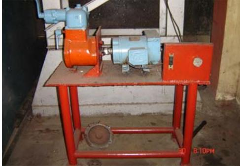
2. Fabrication of small motor resurfacing bench was fabricated by Electrical Component section. With this test bench the armatures of small motors can be re-profiled /polished to remove armature ovality and ensure longer carbon brush life and thus ensure higher reliability on NGC based locos.
