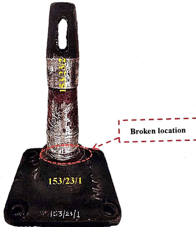
Fig.1 Photograph of broken Center Pivot Pin after joining the received broken pieces.
