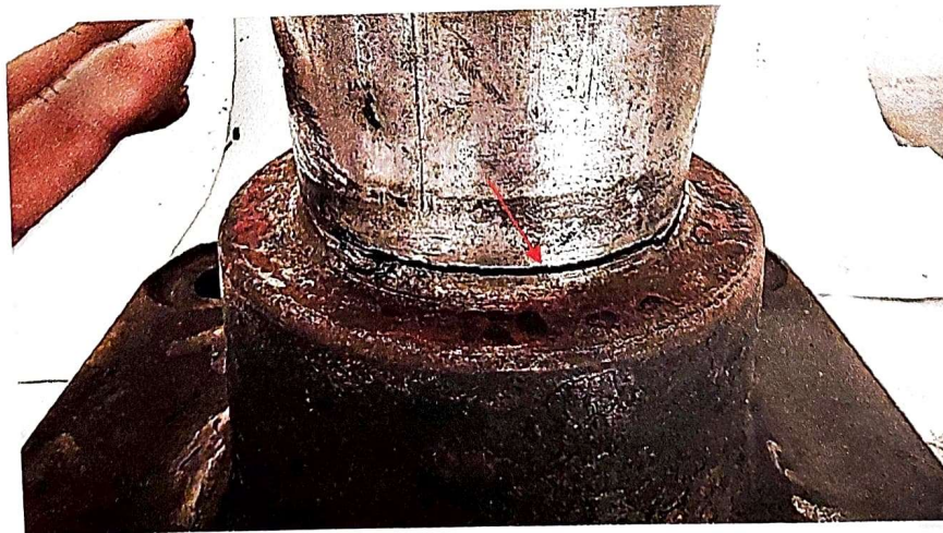
Fig.2 Close view of failed Center Pivot Pin shown in fig.1 above.
