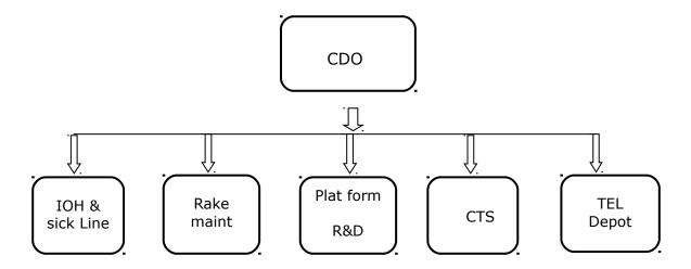
2.3 The central activity of C&W organization of Mechanical department is maintenance of coaching stock and Goods stock. The Key duties consists Rake Maintenance, Intermediate Overhauling, Maintenance at sick line, Receiving and dispatching of trains, Primary and terminal maintenance of rakes.
