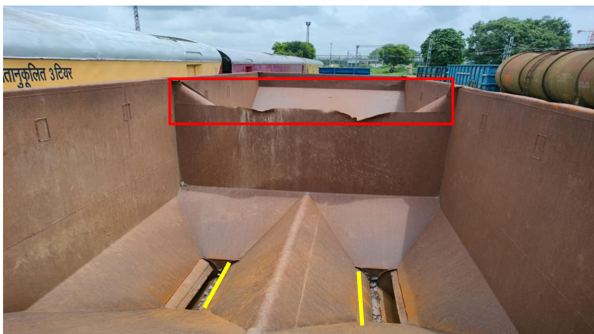
Fig 1- Photograph showing centre door welded (Yellow colour) & damaged partition wall (Red Colour)
