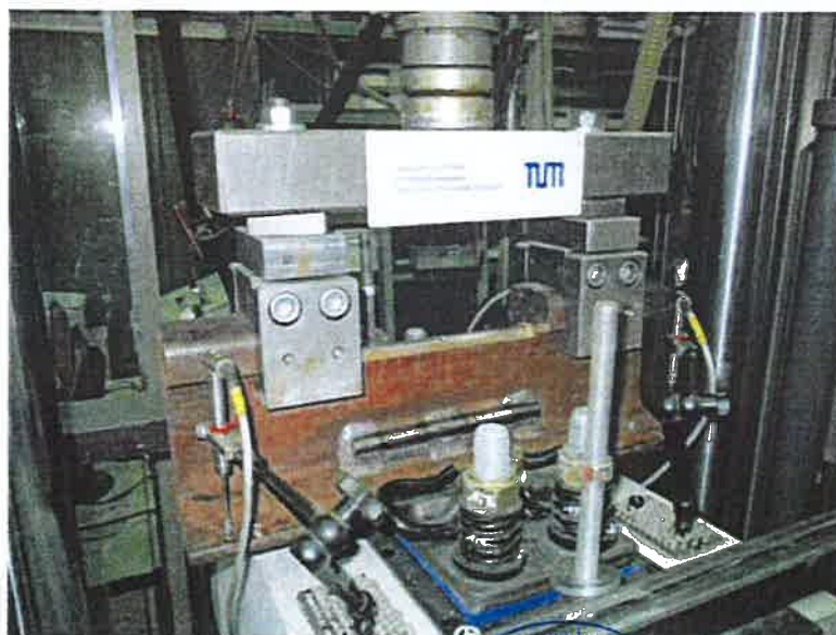
Figure 3: Test rig for the determination of the vertical stiffness of the system
