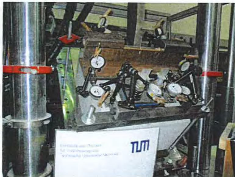
Figure 4: test rig for the repeated load test ( \alpha = 33^\circ ; X^d = 25 \text{ mm} )
