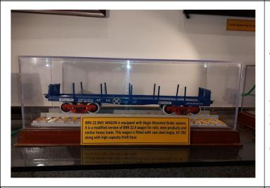
Replica of BRN 22.9 M1 wagon – BRN 22.9M1 Wagon is equipped with Bogie Mounted Brake System. It is a modified version of BRN 22.9 wagon for rails, steel products and similar heavy loads. This wagon is fitted with cast steel bogie, HT CBC along with high capacity Draft Gear.
