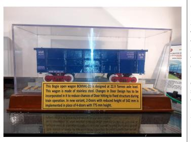
Replica of BOXNHL-2D 22.9 tonnes axle load - The Bogie open wagon BOXNHL-2D is designed at 22.9 Tonnes axle load. This wagon is made of stainless stell. Changes in Door Design has to be incorporated in it to reduce chances of Door hitting to fixed structure during train operation. In new variant, 2-Doors with reduced height of 542 mm is implemented in place of 4-doors with 775 height.
