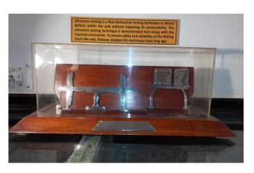
Model of non-destructive ultrasonic testing -
