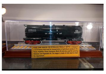
Replica of BTPN 22.9 tonnes axle load wagon -Bogie Tank Wagon Petroleum Product (BTPN) is designed at 22.9 Tonnes axle load for transportation of petroleum products like Petrol, Naphtha, Diesel, Kerosene, Black Oil and also used for carrying Molasses and Vegetable Oil. The wagon is made of mild steel to meet the requirement.
