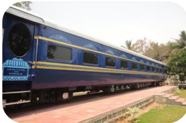
Meter gauge AC library coach NWR 91565 which was running in Palace on wheels train, was brought from N. W. Railway. Its interior, air conditioning was done in LGDS in 2015.
